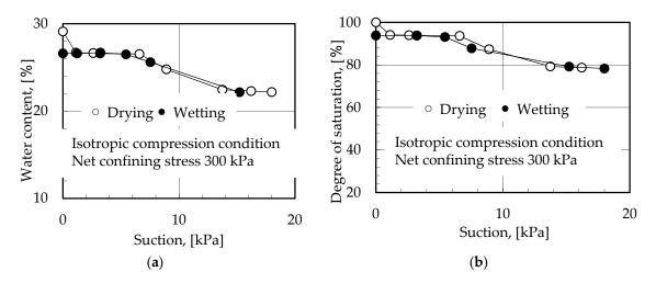
**Figure 8.** Soil—water characteristic curves at 300 kPa net confining stress (**a**) Suction vs. water content at 300 kPa net confining stress; (**b**) Suction vs. degree of saturation at 300 kPa net confining stress.
