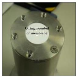
Figure 4. Illustration of Supor 450 saturated microporous membrane on porous stone.
