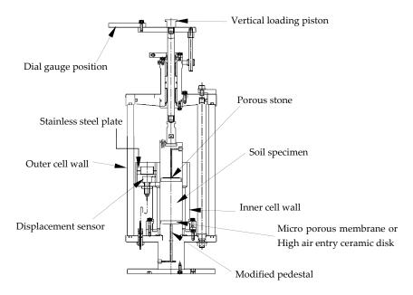
Figure 3. Schematic diagram of modified triaxial apparatus for isotropic stress condition.
