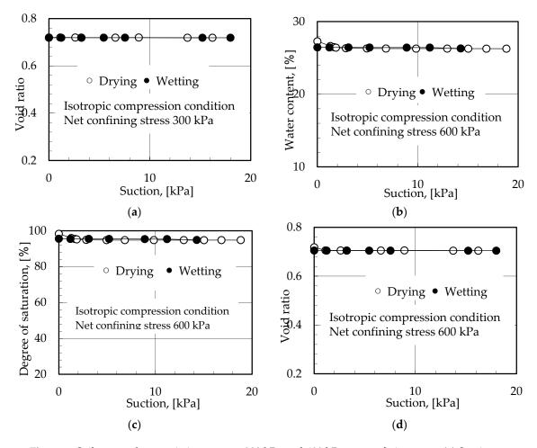
**Figure 9.** Soil—water characteristic curves at 300 kPa and 600 kPa net confining stress (**a**) Suction vs. void ratio at 300 kPa net confining stress; (**b**) Suction vs. water content at 600 kPa net confining stress. (**c**) Suction vs. degree of saturation at 600 kPa net confining stress; (**d**) Suction vs. void ratio at 600 kPa net confining stress.
