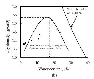
**Figure 1.** Grain size Distribution and compaction curve of silt (a) Grain size distribution for silt soil; (b) Compaction curve for silt soil.
