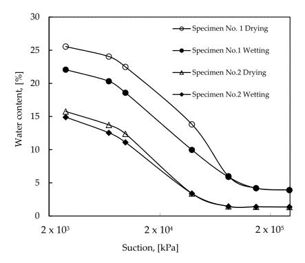
Figure 10. Suction vs. water content for vapour pressure technique data sets.
