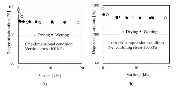
**Figure 6.** Relationship between suction and degree of saturation (a) Suction vs. degree of saturation in one dimensional stress condition; (b) Suction vs. degree of saturation in isotropic stress condition.
