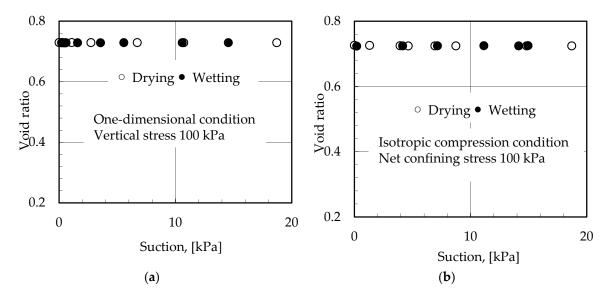
**Figure 7.** Relationship between suction and void ratio (a) Suction vs. void ratio in one dimensional stress condition; (b) Suction vs. void ratio in isotropic stress condition.
