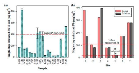
**Figure 2.** Single-step 1 M HNO<sub>3</sub> extracted Pb for (**a**) all samples referenced to the New Jersey Department of Environmental Protection (NJDEP) Residential Direct Contact Soil Remediation Standard (RDCSRS) (400 mg kg<sup>-1</sup>); (**b**) the calculated mean and median of all categories for each site referenced to the background Pb in New Jersey (22 mg kg<sup>-1</sup>) and urban background Pb (111 mg kg<sup>-1</sup>).
