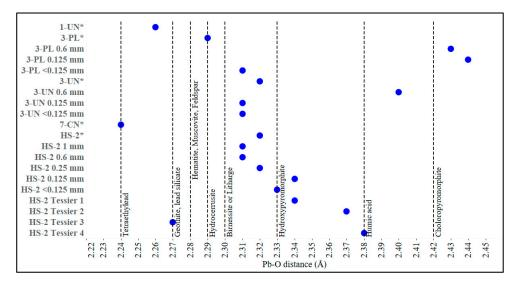
**Figure 5.** First-shell Pb-O distances of samples as determined by X-ray absorption fine structure spectroscopy (XAFS) analysis (y-axis, blue circle) plotted against Pb-O distances of Pb minerals and Pb-mineral sorption complexes (x-axis) as reported in the literature Table S9. Samples marked with an asterisk (\*) are the <2 mm sieved particle size fraction prior to Tessier sequential extraction and sieving to 1 to <0.125 mm particle size.
