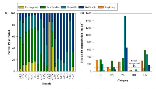
**Figure 3.** Tessier sequential extraction (**a**) normalized to the sum of the total Pb extracted from each fraction; (**b**) median Pb concentration for each step of the sequential extraction and the single-step extraction by sample category referenced to the urban background Pb concentration (111 mg kg<sup>-1</sup>).
