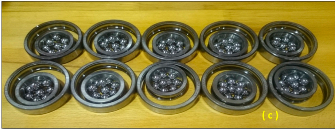
Figure 8. Dismounting of bearings. (a) rivet head removal; (b) epoxy clay mold used to hold the bearing cage; (c) fully dismantled bearings.
