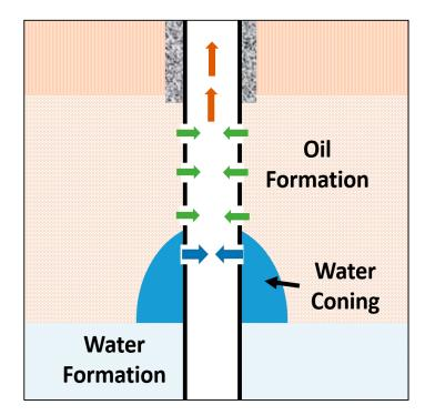
Figure 3. Water coning.
