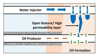
**Figure 1.** Example of a water injection well connected to an oil producer well through an open feature/high permebility layer.
