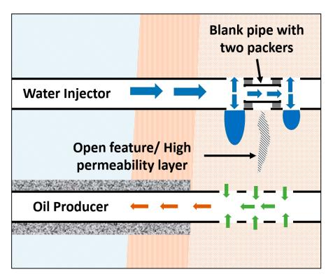
**Figure 8.** Two packers above and below a blank pipe to avoid injecting the water in open features or high permeability layers.
