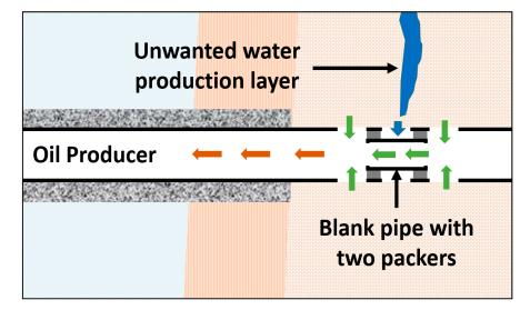
**Figure 7.** Two packers above and below a blank pipe to shut off the production of water from the middle and upper intervals without compromising other oil production zones.
