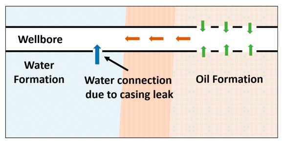
Figure 5. Casing leak connecting the wellbore with water formation.
