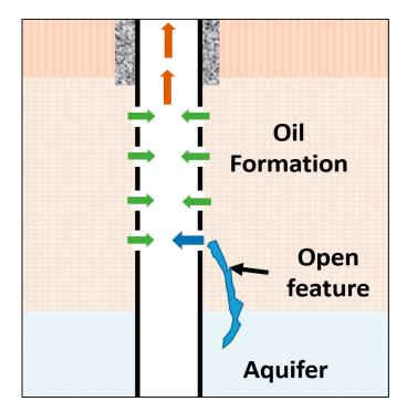
Figure 2. An oil producer connected to an aquifer through an open feature.
