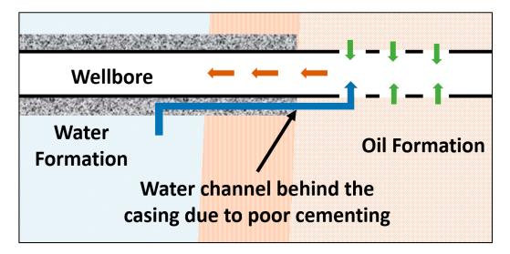
Figure 4. Poor cement behind the casing with a channel connecting water source to the wellbore.
