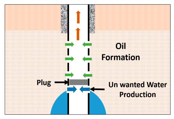
Figure 6. Using a plug to shut off the production of water from the bottom.
