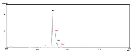
Figure 1. X-ray Flourescence (XRF) of Monel alloy used in the experiments.
