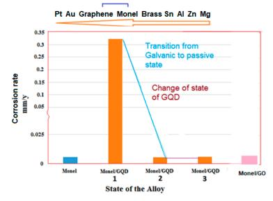
Figure 4. Monel alloy corrosion rates with coatings; 1, 2, 3 represent the polarization measurements.
