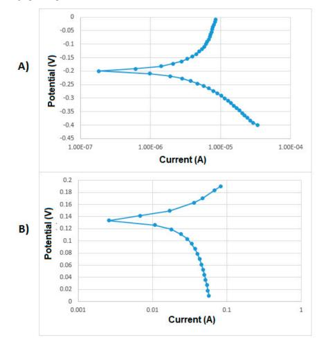
**Figure 3.** Tafel plot and analysis of (**A**) Monel (400) and (**B**) Monel coated with graphene quantum dots for 25 h. Potential is referred with SCE. Medium: 0.1 M NaCl.
