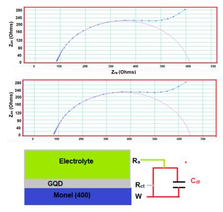
**Figure 6.** Nyquist plot for the Monel coated with Graphene quantum dots (GQD). Upper curve represents first run and bottom curve represents after Tafel polarization. Equivalent circuit is given at the bottom.
