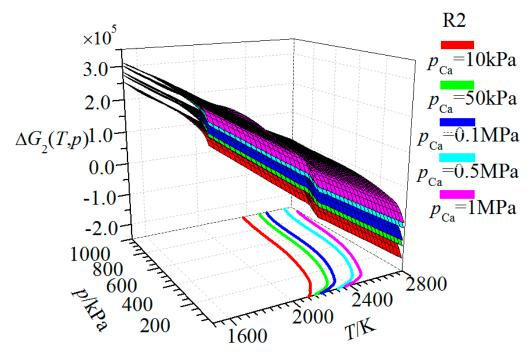
Figure 7. Gibbs energy dependence on temperature and Ca and CO partial pressure for reaction R2.
