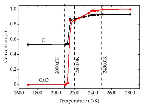
Figure 12. The conversion of C and CaO at each reaction temperature.
