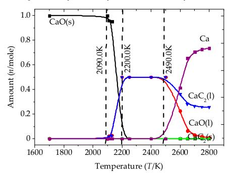
Figure 18. The equilibrium phase composition at each reaction temperature.
