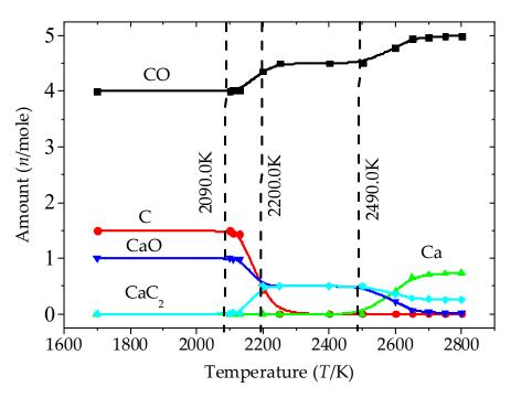
Figure 17. The equilibrium composition at each reaction temperature.
