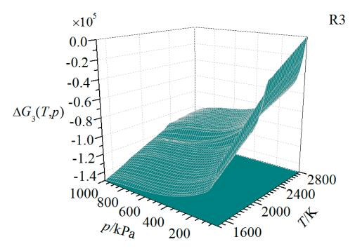
Figure 8. Gibbs energy dependence on temperature and Ca pressure for reaction R3.
