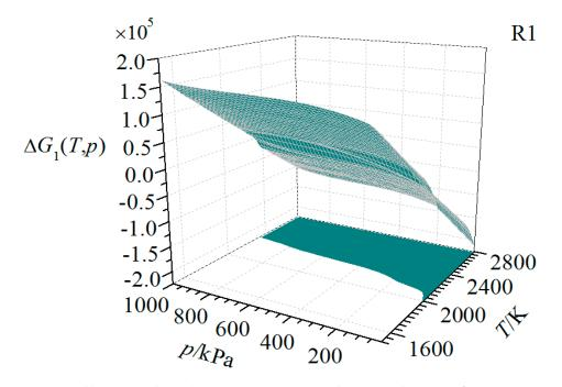
Figure 6. Gibbs energy dependence on temperature and CO partial pressure for reaction R1.
