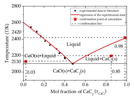
Figure 15. Confirmation of the calculation (Liquid contains CaO (L) and CaC<sub>2</sub> (L)).
