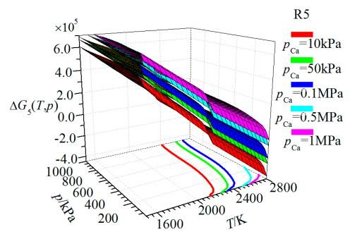
Figure 10. Gibbs energy dependence on temperature and Ca and CO partial pressure for reaction R5.
