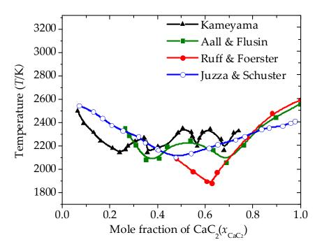
Figure 1. Phase diagram of the CaC<sub>2</sub>-CaO binary system.
