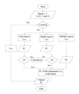
Figure 11. Calculation flow diagrams of the equilibrium components.
