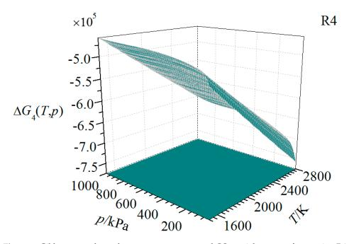
Figure 9. Gibbs energy dependence on temperature and CO partial pressure for reaction R4.
