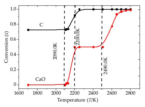
Figure 16. The conversion of C and CaO at each reaction temperature.
