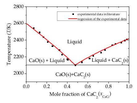
**Figure 2.** Experimental data fitting of phase diagram of CaC<sub>2</sub>-CaO binary system (Liquid contains CaO (l) and CaC<sub>2</sub> (l)).
