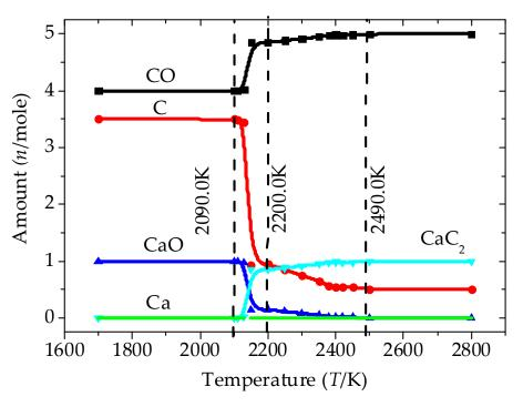
Figure 13. The equilibrium composition at each reaction temperature.
