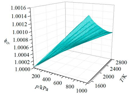
Figure 5. Fugacity coefficient of O<sub>2</sub>.
