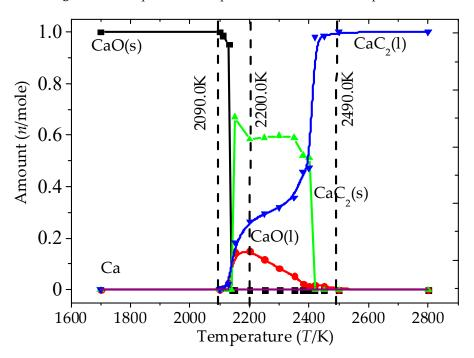
Figure 14. The equilibrium phase composition at each reaction temperature.
