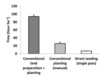
**Figure 1.** Comparison of the average time required for conventional land preparation and conventional planting of maize (land preparation using an animal drawn *maresha* and planting by hand), for conventional planting of maize only (following conventional land preparation), and for direct seeding of maize using a 2BFT-100 seeder powered by a 15 HP two-wheel tractor in an untilled land in Hawassa Ethiopia (source: [23]).
