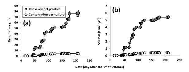
Figure 3. Comparison of (a) the cumulated water runoff and (b) the soil loss for conventional practice and conservation agriculture during the 1994/95 season in Hatcliffe, Zimbabwe, on a Fersiallitic clay soil with a 4.5% slope (source: [26]).
