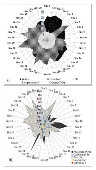
**Figure 4. (a)** Radar plot of water pH, water temperature (°C), and dissolved oxygen (DO), with water temperature and dissolved oxygen varying inversely. **(b)** Radar plot showing concentration (mg/L) of phosphate (PO<sub>4</sub>), cadmium (Cd), zinc ( $Zn^{2+}$ ), copper (Cu<sup>2+</sup>), and sulphide ( $S^{2-}$ ) as measured in water samples.
