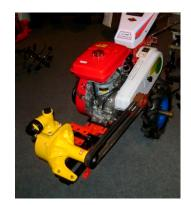
Figure 7. Huaxing 2 WT driving a water pump for crop irrigation (Photo: Brian Sims).
