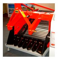
**Figure 10.** Menoble 3-point linkage mounted single row potato harvester for a 30 hp tractor (Photo: Brian Sims).
