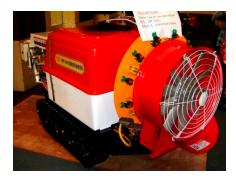
Figure 13. Datang hand-operated, or remote-controlled, fan sprayer for tree crops (Photo: Brian Sims).
