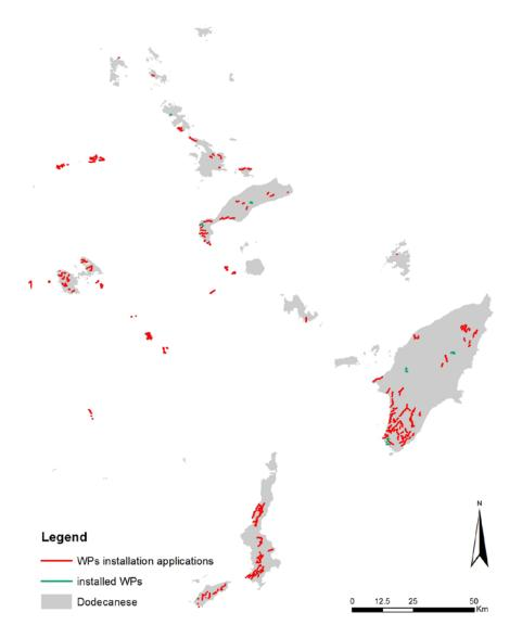
Figure 9. Installed WPs and WPs installation applications for the Dodecanese.
