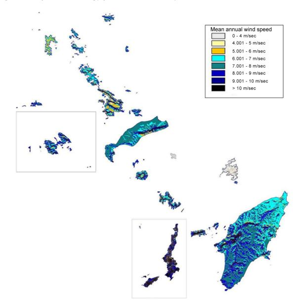
**Figure 7.** Thematic map for the estimation of the technically and economically exploitable potential of wind energy in the Dodecanese islands [59].
