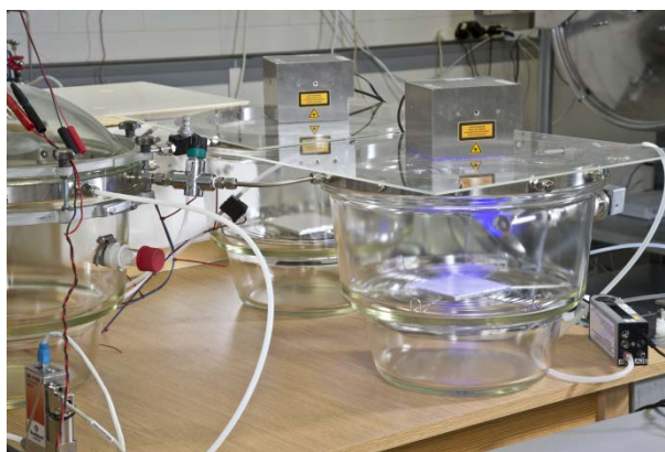
Figure 2. Experimental setup of the gas mixing chamber with two connected 20 L emission test chambers. Both chambers are equipped with ceramic tiles and one is irradiated with UV light.
