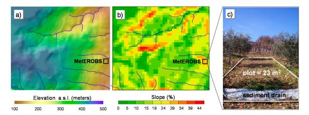
**Figure 4.** Views of (**a**) hillshade-map and (**b**) slope-map at 50 m grid-cell resolution of the Monte Pino experimental site (MPES) with drainage network and MetEROBS (**a**,**b**), and experimental plot placed on the eastern slope of the MetEROBS (**c**).
