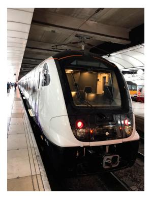
Figure 6. New train with aluminum train compartment.
