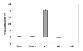
**Figure 3.** Adsorption from aqueous nitrate affected by geomedia and carbon materials. Error bars represent standard error of the mean.
