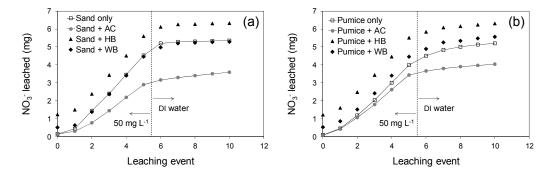
Figure 5. Cumulative amount of nitrate  $(NO_3^{-})$  leached in column effluents: (a) sand and (b) pumice.
