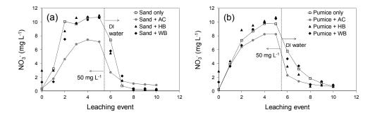
Figure 4. Concentrations of nitrate (NO<sub>3</sub><sup>-</sup>) in column effluents: (a) sand and (b) pumice.
