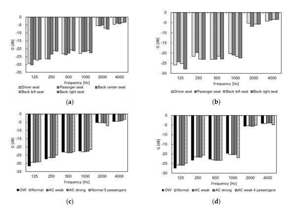
**Figure 3.** Measured *G* [dB] at each passenger position in cars (**a**) A and (**b**) B and under open-window (OW), air-conditioner (AC) and multiple passenger settings in cars (**c**) A and (**d**) B.
