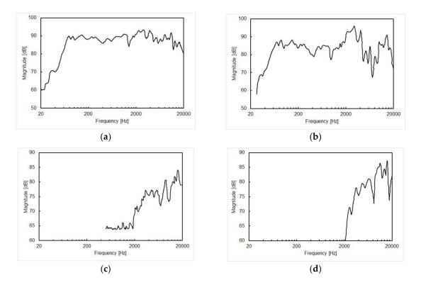
**Figure 2.** Frequency characteristics of the midrange loudspeaker in cars (**a**) A, (**b**) B and the tweeters in cars (**c**) A, (**d**) B.
