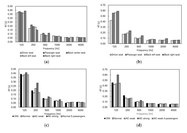
**Figure 4.** Measured reverberation time (*RT*) [s] at each passenger position in cars (**a**) A and (**b**) B and under open-window (OW), air-conditioner (AC) and multiple passenger settings in cars (**c**) A and (**d**) B.
