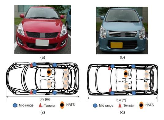
**Figure 1.** Photographs of (**a**) car A, (**b**) car B and the position of the loudspeakers used in the measurements in (**c**) car A, (**d**) car B. The position of the head and torso simulator (HATS) is shown at the driver's position.
