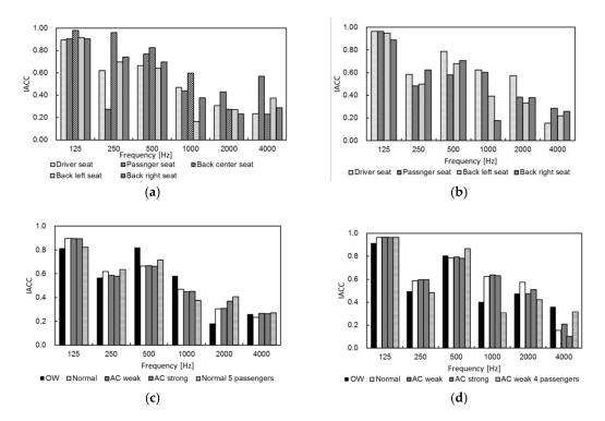
**Figure 7.** Measured inter-aural cross correlation (*IACC*) at each passenger position in cars (**a**) A and (**b**) B and under open-window (OW) and air-conditioner (AC) settings in cars (**c**) A and (**d**) B.
