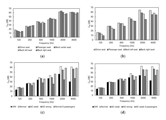
**Figure 6.** Measured  $C_{80}$  [dB] at each passenger position in cars (**a**) A and (**b**) B and under open-window (OW), air-conditioner (AC) and multiple passenger settings in cars (**c**) A and (**d**) B.
