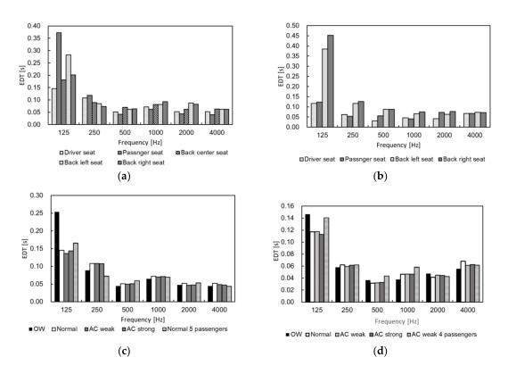
**Figure 5.** Measured early decay time (*EDT*) [s] at each passenger position in cars (**a**) A and (**b**) B and under open-window (OW), air-conditioner (AC) and multiple passenger settings in cars (**c**) A and (**d**) B.
