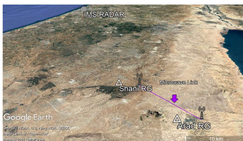
Figure 1. The experimental setup: the location of the weather radar, the CML, and the two Rain Gauges (Arad and Shani) are marked. This image is copied from [23], where the same experimental setup was used for a different purpose.
