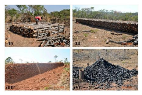
**Figure 2.** Processes of charcoal production by traditional earth kiln. Upper images (**II**) show the process of log piling into clamp, and the lower left image (**III**) shows covering of the clamp with dung and soil lumps, while the lower right image (**V**) shows the harvesting of charcoal and packaging it into bags. The steps number (**I**,**IV**) are not represented in this figure.
