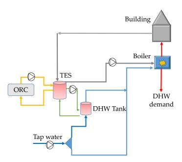
Figure 3. Space heating (SH) and domestic hot water (DHW) plant configuration.
