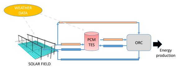
Figure 2. Conceptual schematics of the micro-solar organic Rankine cycle (ORC) plant.
