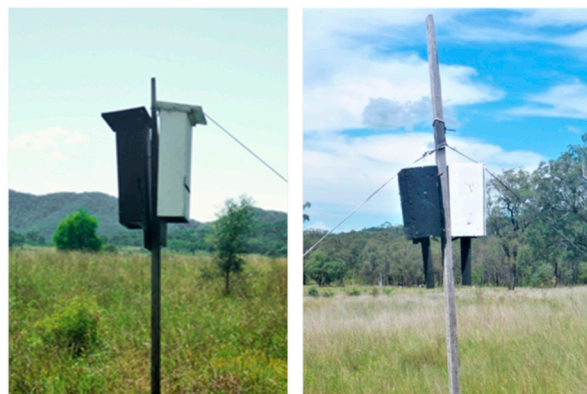
Figure 1. Paired plywood design ( left ) and paired wood-cement design ( right ) installed on poles about 1.5 m above ground.
