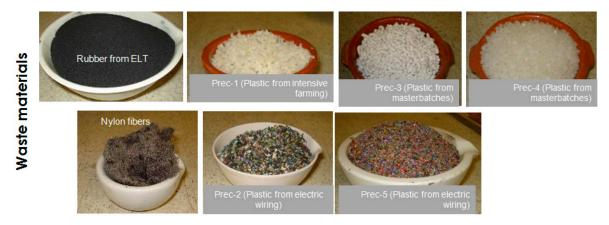
Figure 5. Materials used for generating the additives for asphalt mixes.
