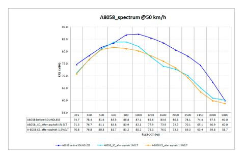
**Figure 11.** Average spectrum obtained on the A-8058 test track before and after paving the LIFE SOUNDLESS mixtures.
