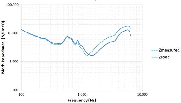
Figure 8. Impedance measurement and the mechanical impedance estimated for the road.
