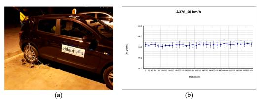
**Figure 4. (a)** Image of the self-propelled vehicle used for the close proximity (CPX) measurements. (b) Results of CPX\_*p* at the A-376 site at 50 km/h.
