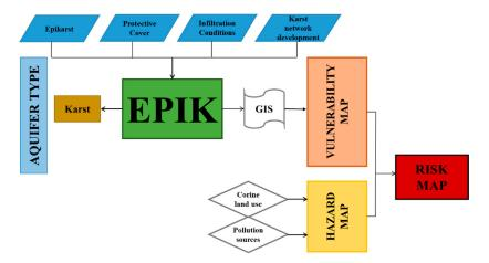
Figure 4. Flowchart of the used processes for generating the vulnerability and pollution risk maps.
