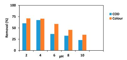
**Figure 2.** Effect of pH on photocatalytic degradation (process conditions: TiO<sub>2</sub> dosage—500 mg/L, reaction time—3 h, UV light irradiation—64 W).
