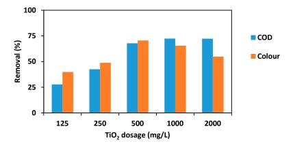
**Figure 3.** Effect of catalyst dosage on photocatalytic degradation (process conditions: pH—4, reaction time—3 h, UV light irradiation—64 W).
