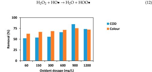
**Figure 6.** Effect of oxidant dose on photocatalytic degradation (process conditions: pH—4, reaction time—3 h, UV light irradiation—64 W, catalyst dose—500 mg/L).
