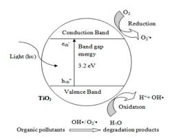
**Figure 1.** Photocatalytic mechanism for TiO<sub>2</sub> photocatalyst.
