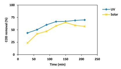
**Figure 7.** Influence of incident irradiance on COD removal over the 3.5-h duration test (process conditions: pH—4, UV light irradiation—64 W, catalyst dose—500 mg/L).
