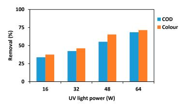
**Figure 4.** Effect of UV light irradiation power on photocatalytic degradation (process conditions: pH—4, reaction time—3 h, TiO<sub>2</sub> dosage—500 mg/L).
