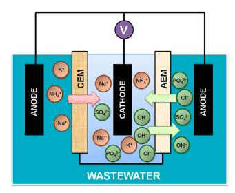
**Figure 6.** Schematic diagram of Removing-Recovering Bio-Electrochemical System (R<sup>2</sup>-BES) for recovery of nitrogen and phosphorus from wastewater. Abbreviations: CEM (cation exchange membrane); AEM (anion exchange membrane). Adapted from the ref. [102].
