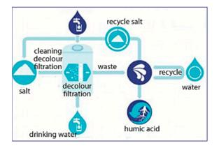
**Figure 4.** Process flow diagram of the HumVi technology to recover humic acid from wastewater. Adapted from ref. [75].
