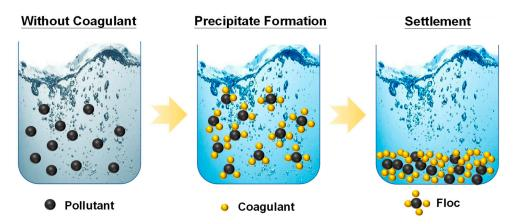
Figure 3. Principles of chemical coagulation used for removing colloidal pollutants in wastewater.
