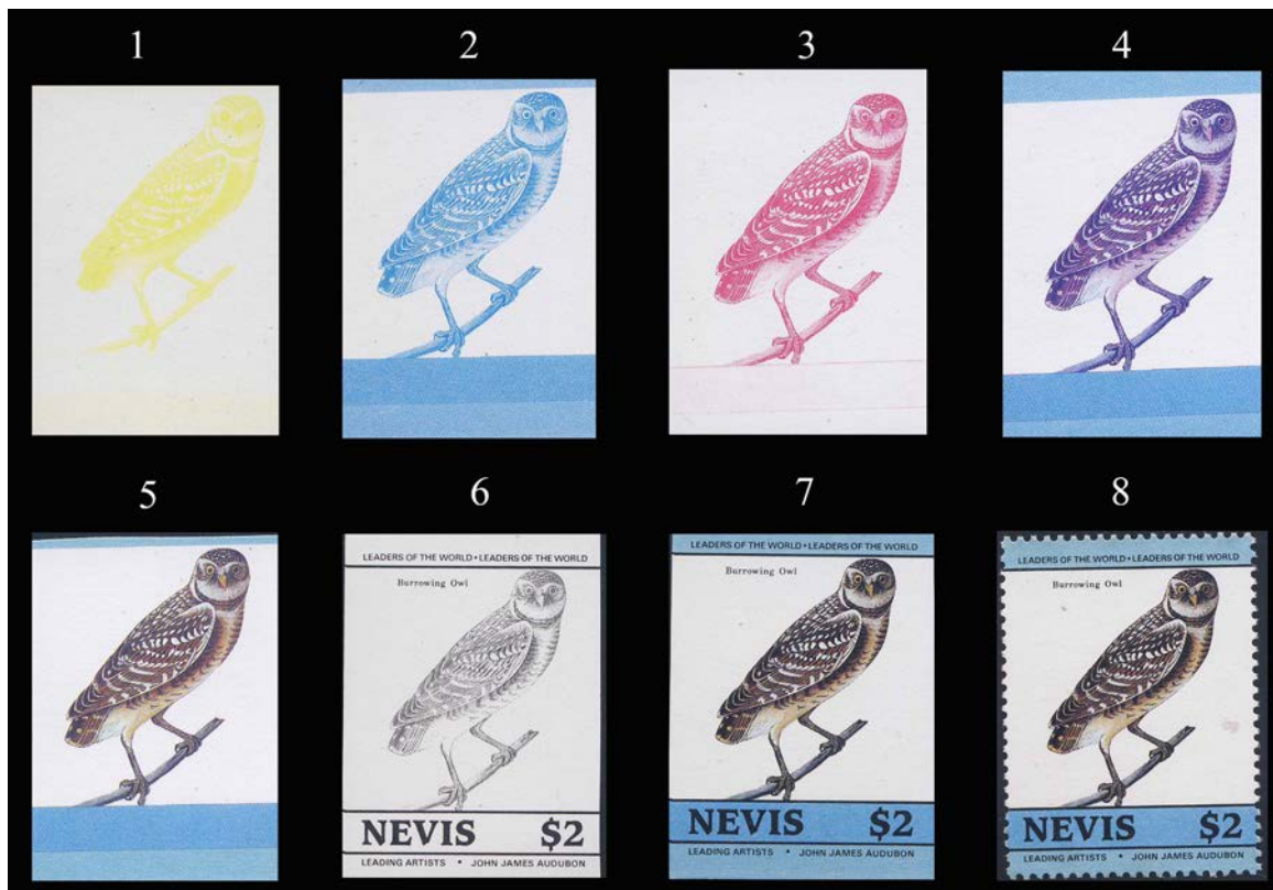
Image 11. 'Printer's Proofs' and 'Progressive Printer's Proofs'. Once the printing process begins, images are prepared, each image devoted to a separate colour. In the beginning the three primary colours, viz. yellow, cyan and red (1, 2 and 3) are prepared, and impressions taken by the printers for checking – hence these are called 'Printer's Proofs'. Then, these are superimposed upon one another (4) to see the effect and determine whether additional colours are necessary. In this case it was decided to use brown. (5). Finally, black was used along with the country's name (6) and the final result achieved (7). Impressions are taken at all stages by the printers, and these are termed 'Progressive Printer's Proofs' or 'Progressive Proofs'. After perforation, the stamp depicting the Burrowing Owl Athene cunicularia was issued (8).
