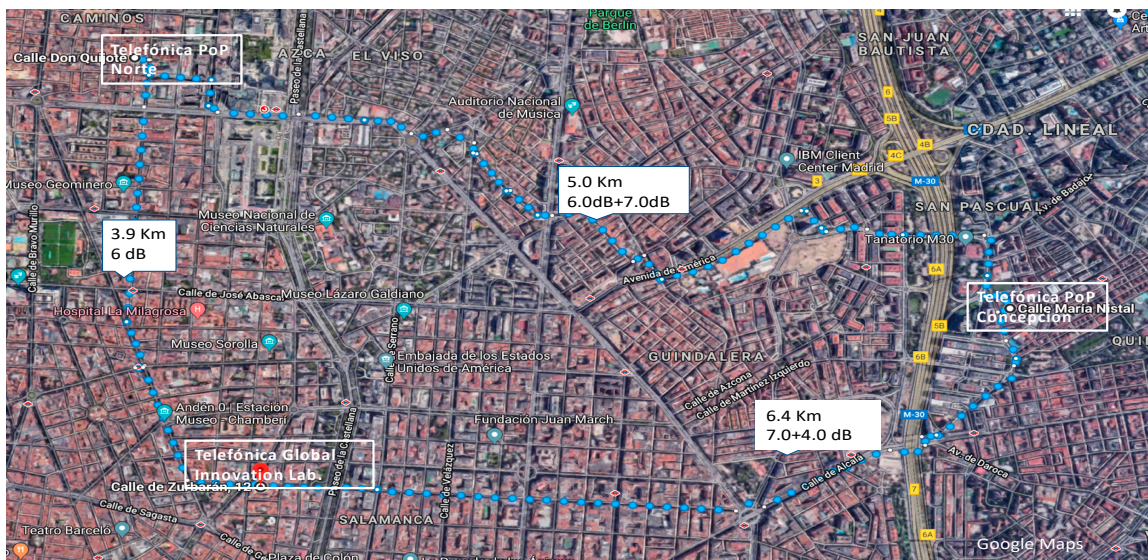
Figure 1. Physical topology of the three nodes used in the reported demonstrator.
