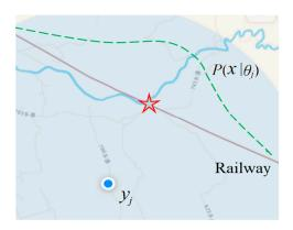
**Figure 4.** Illustrating a GPS device's positioning with a deviation. The round point is the pointed position, the star is the most possible position, and the dashed line is the predicted probability distribution. Source: author.
