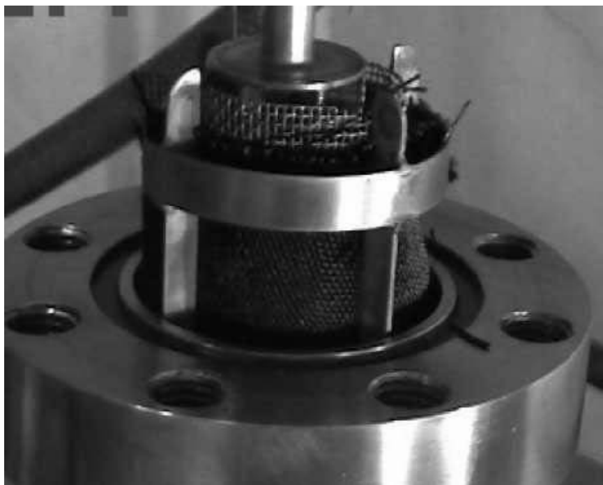
Figure 2 Experimental setup for liquid phase reaction with ACC catalysts (the grid supporting the ACC is partially lifted out of the autoclave).
