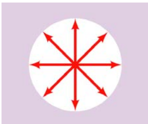
Figure 5.10 Oscillation of the electrical field of ordinary light occurs in all possible planes perpendicular to the direction of propagation.
