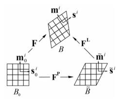
Fig. 3.9 Crystal plasticity kinematics
