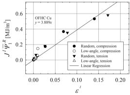
**Fig. 9.2** Results from crystal plasticity simulations of uniaxial tensile and compressive deformations of polycrystalline copper (Clayton and McDowell 2003a). A scalar measure of the magnitude of residual lattice strain is  $\varepsilon^I$ , and stored energy per unit intermediate volume associated with residual lattice strain is  $\overline{\Psi}_1^R$ .
