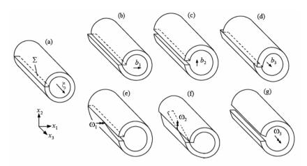
Fig. C.2 Volterra's line defects: defect line (a); edge dislocations (b), (c); screw dislocation (d); twist disclinations (e), (f); wedge disclination (g)
