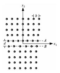
Fig. C.5 Edge dislocation in a cubic lattice
