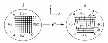
Fig. 3.15 Defective cubic lattice as described by the crystal connection
