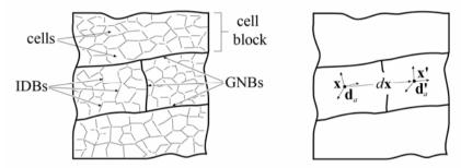
**Fig. 3.18** Dislocation substructure (left) and lattice director vectors (right) in a severely plastically deformed (SPD) single crystal
