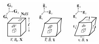
**Fig. 3.12** Configurations, local volumes, and coordinate systems in reference configuration  $B_0$ , intermediate configuration  $\overline{B}$ , and current configuration B
