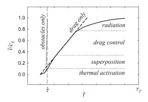
Fig. 6.1 Dislocation velocity-shear stress diagram (Kocks et al. 1975)
