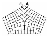
Fig. 3.17 Full negative (90°) wedge disclination in cubic lattice (Lardner 1974)
