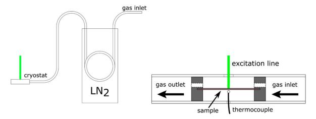
**Figure 2.** The experimental setup for study of Raman spectrum of KAgF<sub>3</sub> at low temperature.
