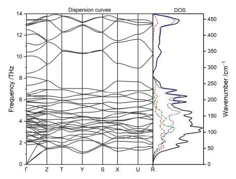
**Figure 5.** The calculated phonon dispersion and phonon (atomic) density of states for KAgF<sub>3</sub> (blue dotted line—F, red dashed line—Ag, green dash-dotted line—K).
