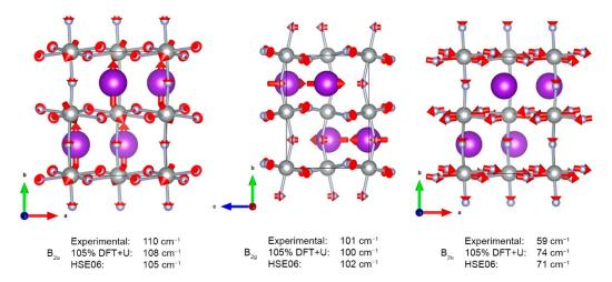
Figure 6. Normal vectors for selected fundamentals. Red arrows show the direction and relative amplitude of atomic movement.
