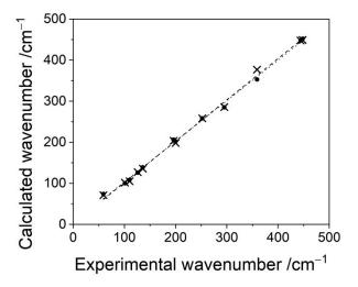
**Figure 7.** Correlations between theoretical and experimental wavenumbers jointly for IR and Raman spectra (black dotted line—linear regression with  $R^2 = 0.999$  for corrected DFT+U dataset, black dashed line—linear regression with  $R^2 = 0.997$  for HSE06 dataset; both not bound to pass at (0,0)).
