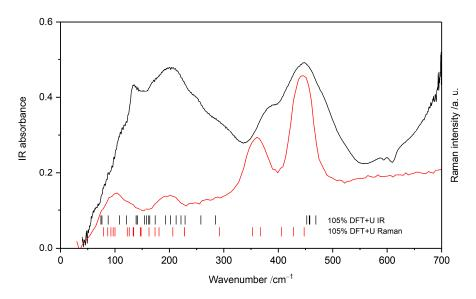
**Figure 3.** FIR (black) and Raman (red) spectra of KAgF<sub>3</sub> at room temperature together with marks indicating the computed wavenumbers.
