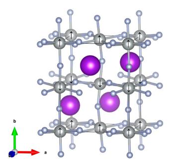
**Figure 1.** Ground state spin ordering in KAgF<sub>3</sub> *P*nma structure as marked by black arrow (gray—Ag; light blue—F; violet—K).
