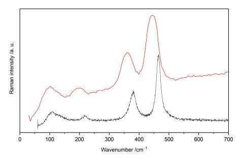
Figure 4. Raman spectrum measured at room temperature (red) and 123 K (black).
