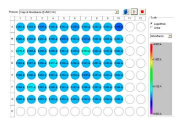
Figure 2. A sample image of spectrophotometric assay obtained by a VICTOR<sup>TM</sup>X4 microplate reader.
