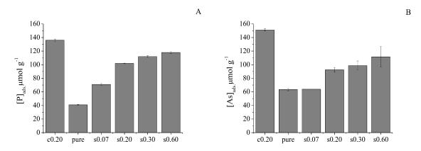
Figure 5. Comparison of phosphate and arsenate sorption on Zn-sorbed and 0.2Zn co-precipitated  $\delta$ -MnO<sub>2</sub> (error bars represent results from duplicate experiments). "c" stands for "Zn-coprecipitation" samples and "s" for "Zn-sorption" samples. Initial phosphate and arsenate concentrations are 100 μM.
