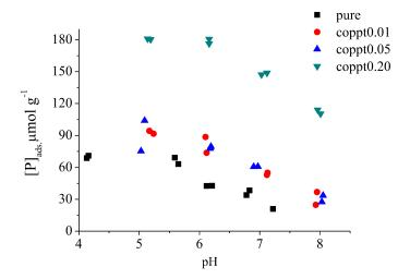
**Figure 4.** Phosphate sorption on pure, coppt0.05, and coppt0.20  $\delta$ -MnO<sub>2</sub> samples as a function of pH. Initial phosphate concentration is 100  $\mu$ M.
