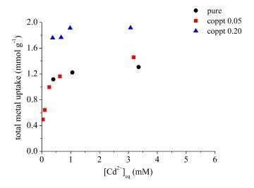
**Figure 2.** Total metal uptake (calculated by Equation (1)) on pure and Zn-coprecipitated  $\delta$ -MnO<sub>2</sub> samples.
