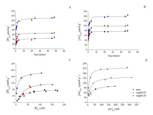
Figure 3. (A) Phosphate and (B) arsenate sorption kinetics on pure, coppt0.05, and coppt0.20  $\delta$ -MnO<sub>2</sub> samples. Solid lines are pseudo first order model fitting results. (C) Phosphate and (D) arsenate sorption isotherms on pure, coppt0.05, and coppt0.20  $\delta$ -MnO<sub>2</sub> samples. Initial phosphate and arsenate concentrations are 100 μM. Solid lines show the Langmuir fitting results. Error bars represent results from duplicates.
