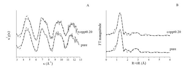
**Figure 6.**  $k^3$ -weighted As extended X-ray absorption fined structure (EXAFS) spectroscopy (**A**) and Fourier transformed spectra (not corrected for phase shift) (**B**) of arsenate sorption on pure and coppt0.20 δ-MnO<sub>2</sub> samples. Raw and fitted data are in solid and dotted lines, respectively.
