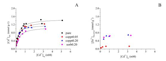
Figure 1. (A)  $Cd^{2+}$  sorption isotherms on pure, Zn-coprecipitated (coppt0.05, coppt0.20) and Zn-sorbed (sorb0.20) δ-MnO<sub>2</sub> samples. (B) Amount of Zn<sup>2+</sup> release (desorption) during  $Cd^{2+}$  sorption. Solid lines are Langmuir model fitting results.
